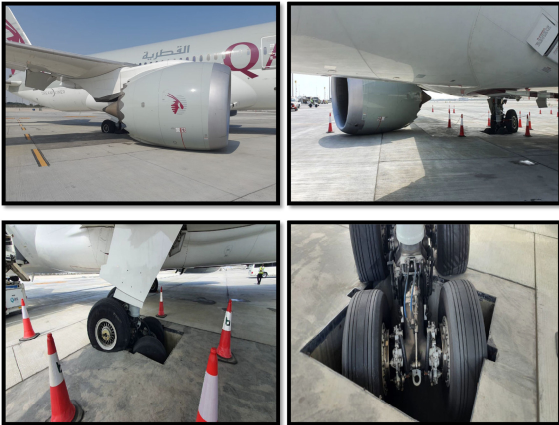
Figure 1: A view of the aircraft, the right-side main landing gear assembly, and No 2 Engine touching the ground – from different perspectives.
